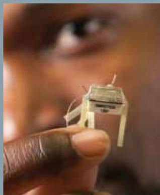
Dzirasa holds the special micro-array helmet worn by mice in his lab. Electrodes in the helmet record brain patterns in real time.
