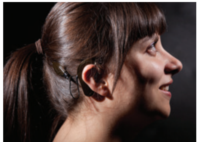
The external portion of the implant includes a microphone and sound processor worn behind the ear and a transmitter held in place by a magnet.
