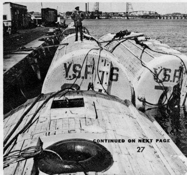
Salvage pontoons which will raise the Squalus from the bottom are 32 ft. long and 13 ft. in diameter.
