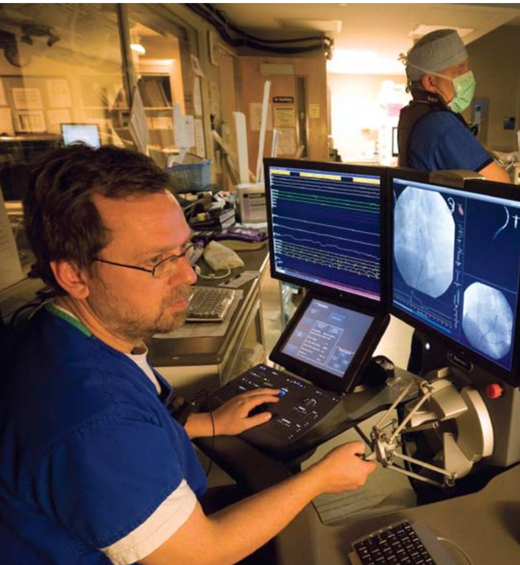
Tristram Bahnon, MD, uses a Hansen Medical Sensei X Robotic Catheter System that allows catheters to be manipulated with greater control and precision within the heart. Outcomes research is under way at Duke to establish the value of this system and develop it further.
