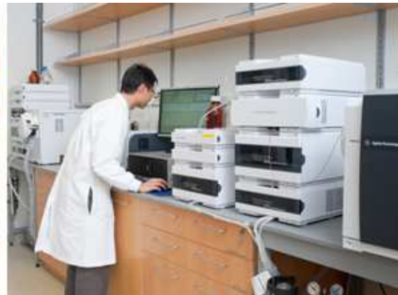
The triple quadrupole liquid chromatography-mass spectrometer separates compound mixtures, which are then used to analyze more polar compounds.
