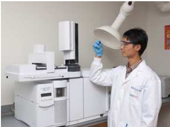
The gas chromatography-mass spectrometer separates volatile compound mixtures then detects the compounds by creating a mass spectrum of each compound.
